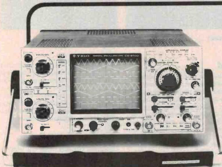
**TRIO's CS2100 100MHz scope** has the capacity to provide 4 channel/8 trace displays with completely independent A and B sweeps ... sensitivity of 1mV/div right up to 100MHz ... observe fast signals with a max sweep speed of 2nS/div ... select 50ohm or 1Mohm inputs ... separate intensity controls for delayed and main sweeps to maintain brightness ... autofocus and 16kV post acceleration CRT ... weighs only 7.5kg - truly portable.
